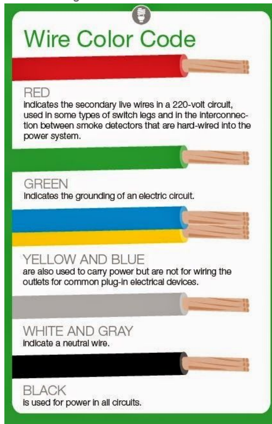
Figure 19. Wire Color Code
